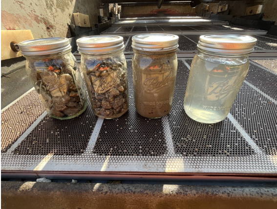
Recycled output: aggregate grades & reclaimed water
